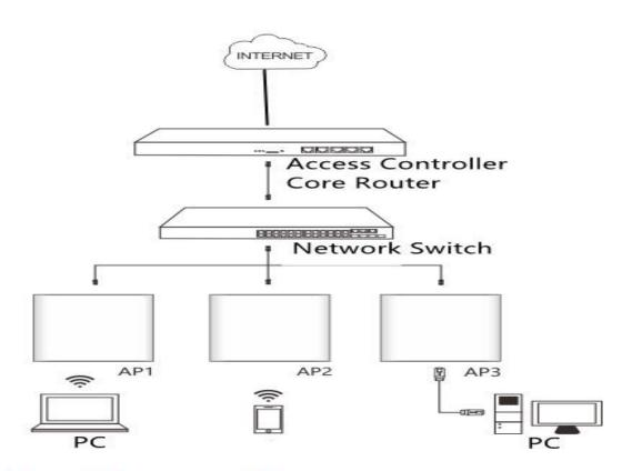
AC routing mode: as a router and access controller
